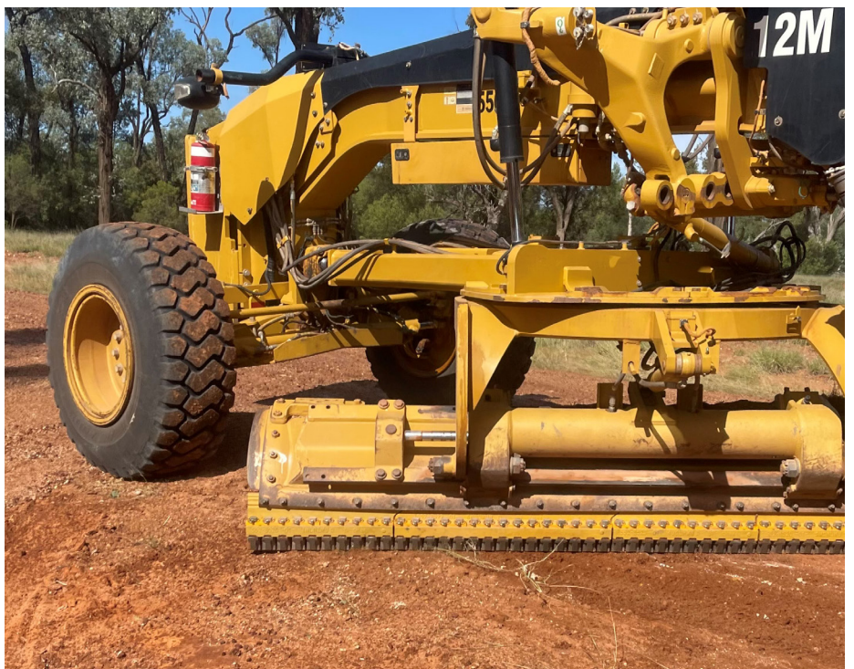
The new technology replaces two grader blades with 70 nickel carbide teeth, which can be individually replaced as wear occurs.
